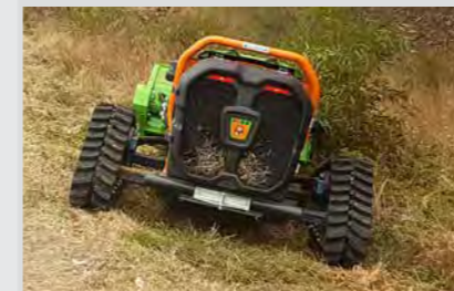
WIDENING TRACKS +400mm
